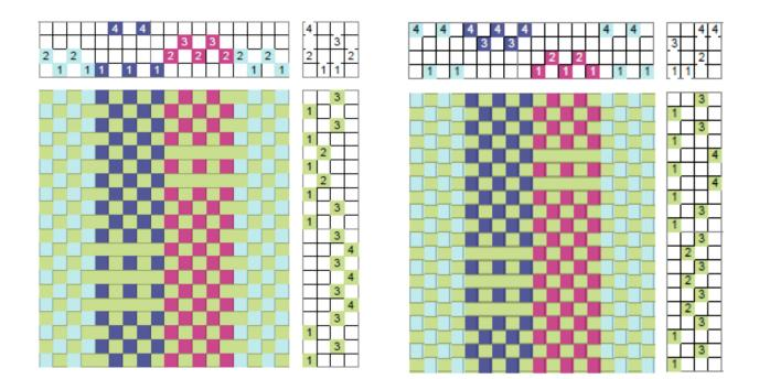
The reason that the drawdown on the left is used more often it's because it is easier to expand it to more shafts: shafts 1 and 2 can be also used for other blocks; for example, the next block, C, uses shaft 2 and 5; block D uses shafts 1 and 6, etc. The odd and even sequence is always maintained since this is, after all, a structure derived from plain weave.
