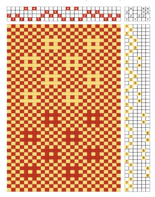
In contrast, the drawdown of Bronson Lace below shows that all of the blocks can be woven together with the same type of floats. This characteristic is the result of the blocks being independent, all using the same tie-down thread, causing the structure to be classified as a unit weave (Robin Spady uses a slightly different characteristic to classify the structure as unit).
